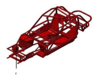
Diagram of chassis showing the position at which ride height measurements will be taken, front (F) and rear (R).
