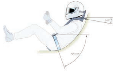
Figure 14 recommended belt angle for open cockpit cars
